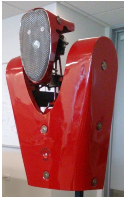
Figure 3.6: MARVIN’s inherited actuated humanoid torso.
