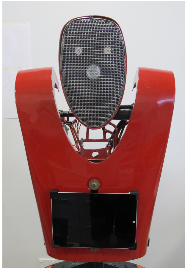
Figure 3.10: Surface 3 Pro, mounted on MARVIN's torso.
