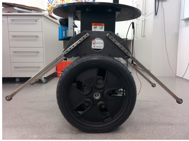
Figure 3.2: Segway RMP augmented with tilt limiters [3].
