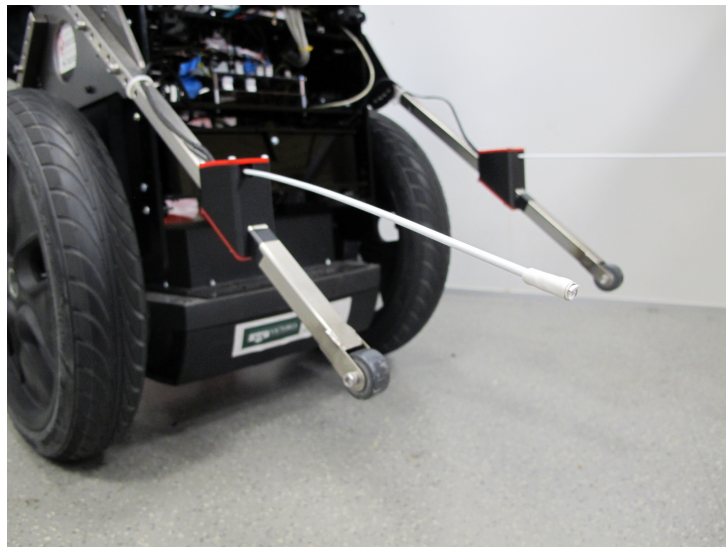
Figure 3.8: Whisker sensors mounted on MARVIN's front tilt limiters.
