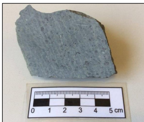
Figure 4.23. Flow banding texture of andesite at WK-122/584 m.
