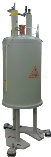
Figure 3.19: Bruker Wide Bore 400 MHz superconducting magnet (spectrometer and operator console are not shown).
