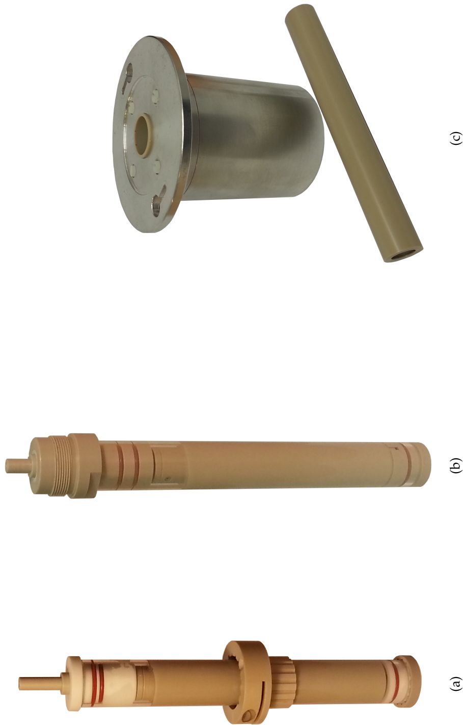
Figure 5.1: Various concentric cylinder shear devices. (a) Variable temperature variant compatible with Magritek Rheo-NMR system (bayonet connection); the end caps of this device are machined from MACOR®. (b) Zero backlash variant which couples via threaded connection to housing of drive-shaft unit. (c) Accessory developed for TA Instruments AR 2000 rheometer.
