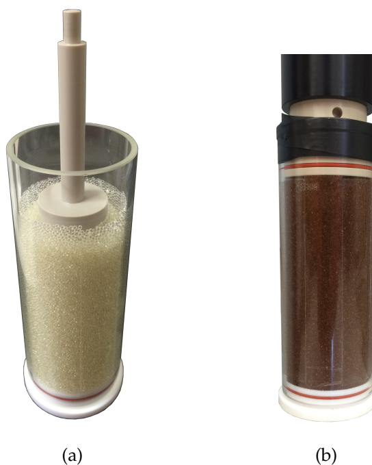
Figure 7.7: (a) Vitamin E capsules loaded in a concentric cylinder shear device (top cap not installed). The layer of seeds affixed to the glass tubing is visible at the top of the fluid domain. (b) Shear device loaded with lobelia seeds and mounted to super wide bore drive-shaft unit; electrical tape was used to prevent slip between the cap of the concentric cylinder and the glass tubing.
