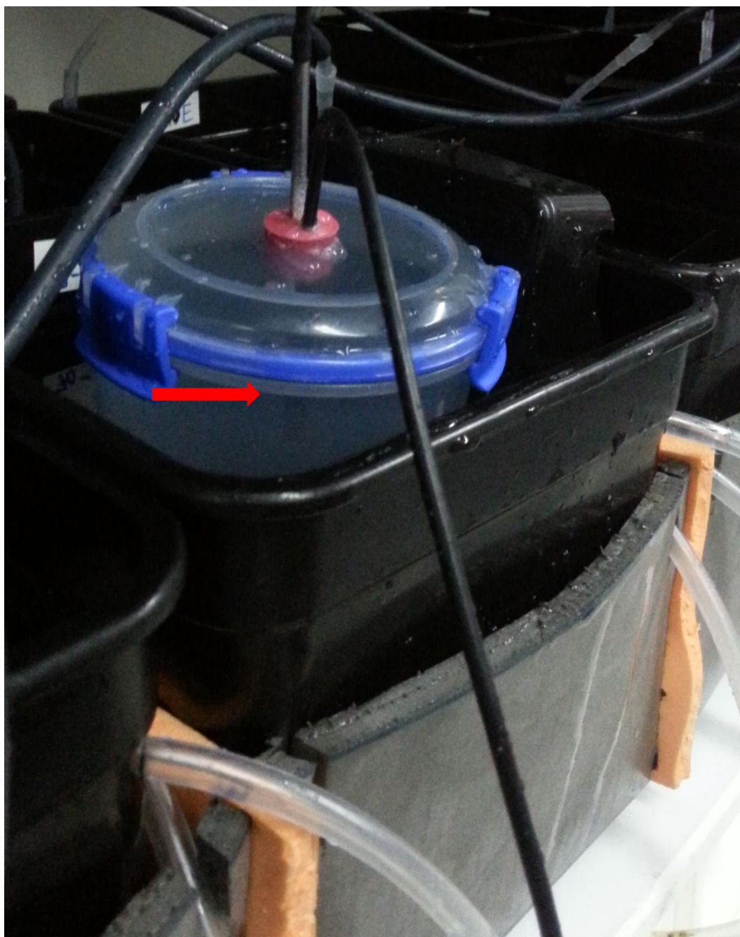
Figure 2.8 - Respiration chamber in a water bath , with measurements underway. Most of the respiration chamber is submerged in the water bath of treatment-specific temperature to keep its temperature stable. The water bath level extends nearly to the lip of the chamber; the water-line in the water bath is indicated by a red arrow.
