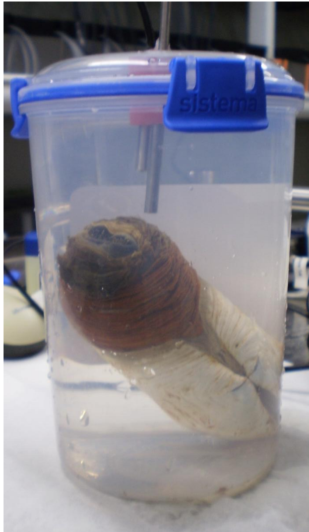
Figure 2.6 - Closed 1 L respiration chamber containing Laternula elliptica . Temperature and O 2 fibre optic probes (grey rods) are visible inserted into the chamber.
