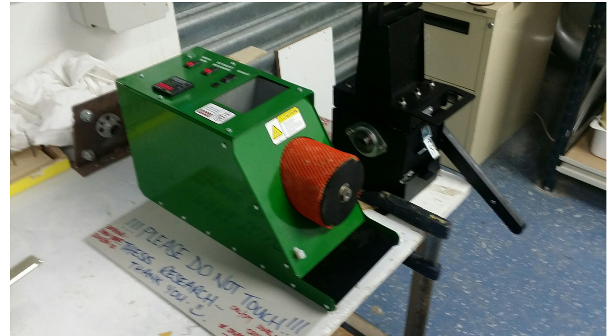
—Figure 26 Filament extrusion lab. FilaBot Original® and FilaBot Reclaimer®. Setup in the School of Design Workshop, VUW (image by Lionel Taito-Matamua)
