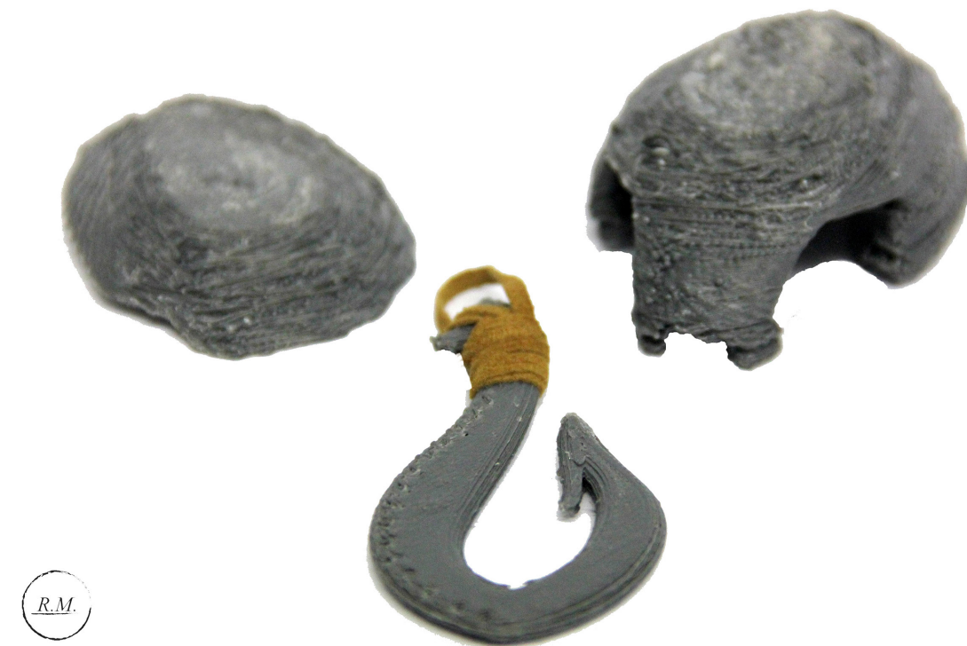
-Figure 36 3D printed Pacific inspired hook and partial printed Turtle skulls made out of recycled ABS filament. Finished with lashed leather. (image by Lionel Taito-Matamua)
