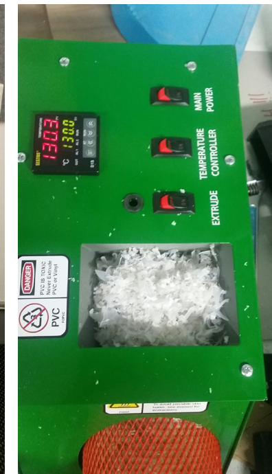
–Figure 28 Reclaimed HDPE particles placed into the hopper (image by Lionel Taito–Matamua)
