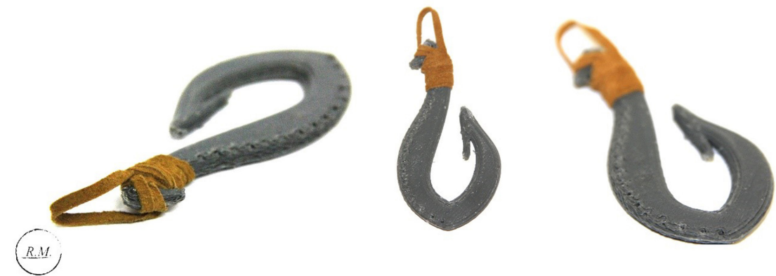
-Figure 35 3D printed Pacific inspired hooks made out of recycled ABS filament. Finished with lashed leather. (image by Lionel Taito-Matamua)
