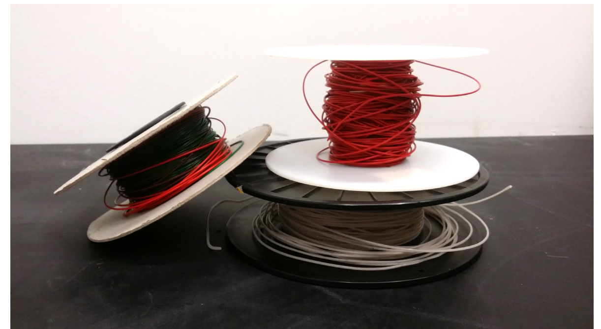
–Figure 30 Recycled Filament made using the extrusion lab. Colours were added using ABS colourants. (image by Lionel Taito–Matamua)
