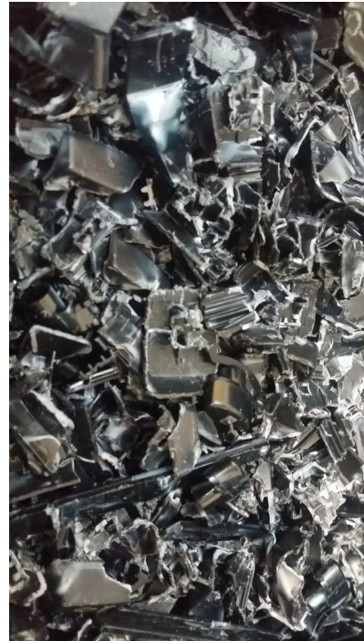
-Figure 31 ABS Keyboard, shredded using the reclaimer. (image by Lionel Taito-Matamua)
