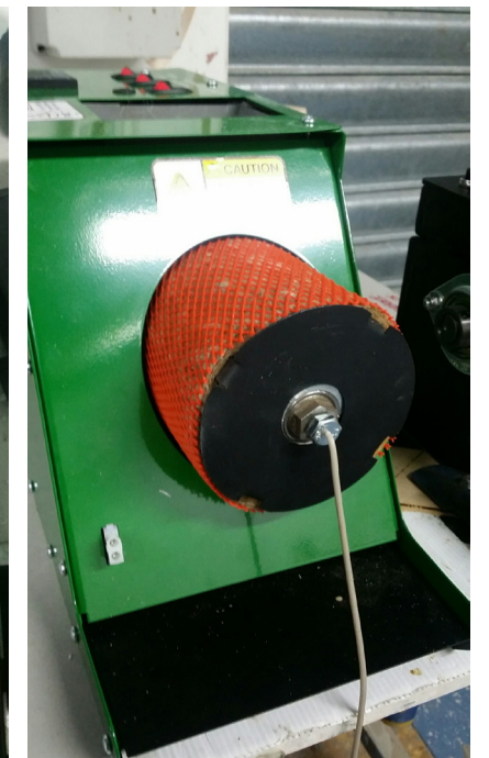
–Figure 29 Recycled HDPE filament being extruded. (image by Lionel Taito–Matamua)
