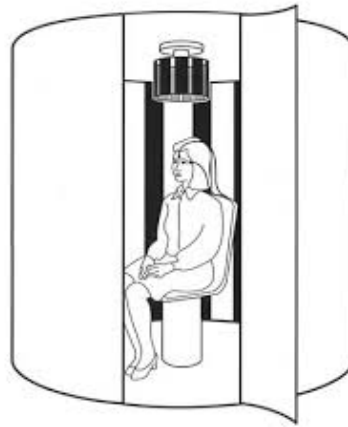
Figure 2.3: An optokinetic drum. The drum's interior is vertically striped, so when the drum rotates, a person sitting inside the drum is subjected to a moving visual field while they remain stationary.
