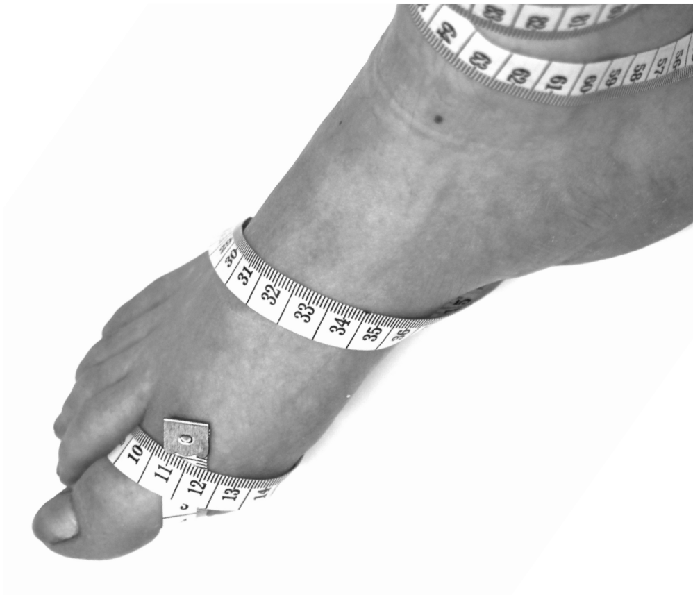
Figure 4.45 - Tape measure wrapped around foot to determine sensor positions
