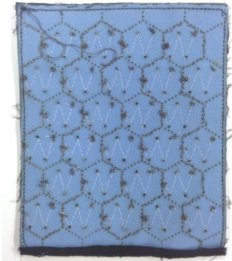
Figure 4.3 - Sensor mat with 27 velostat sensors
