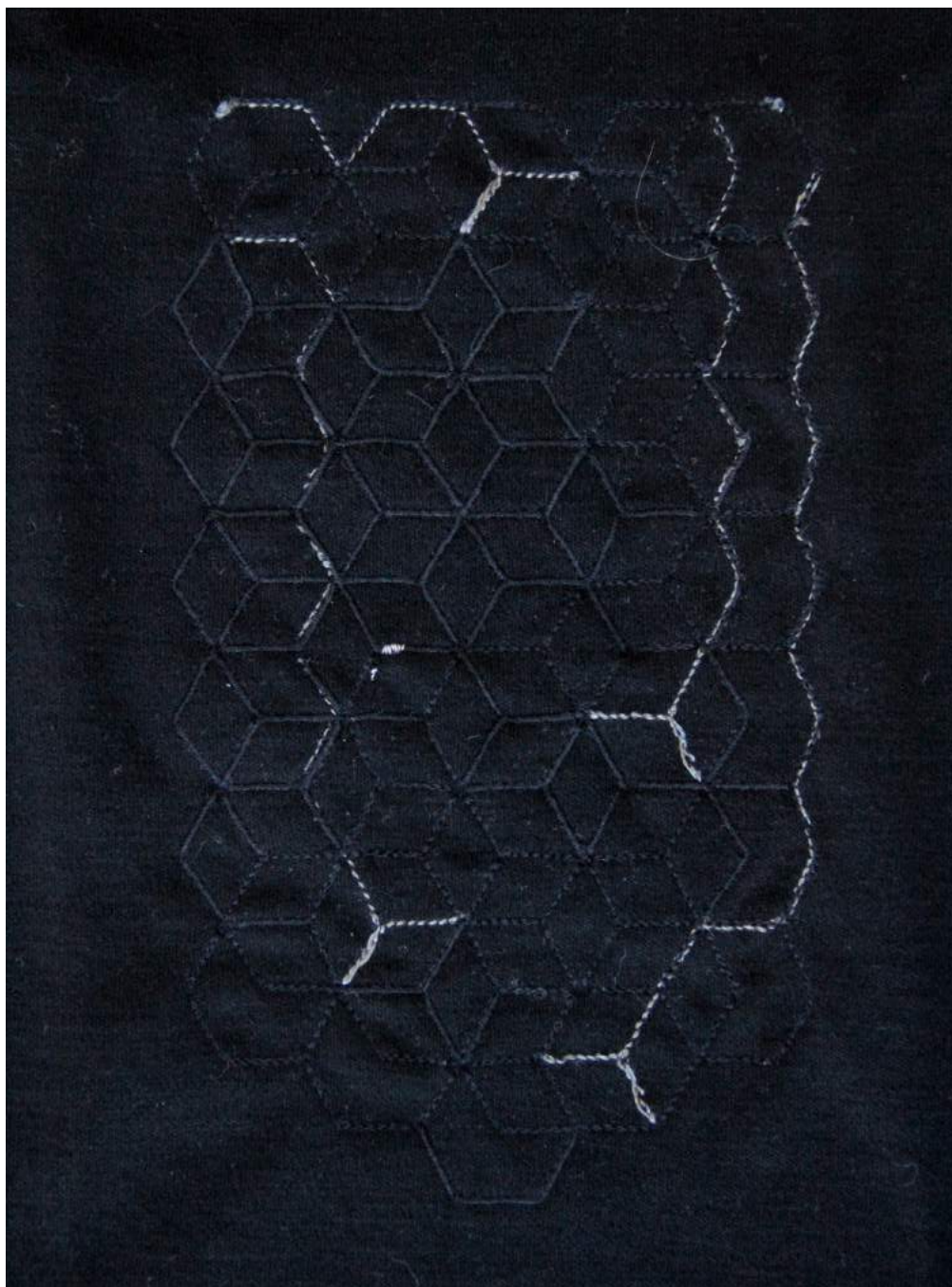
Figure 4.38 - Hexagon pattern with conductive tracks covered in satin stitch
