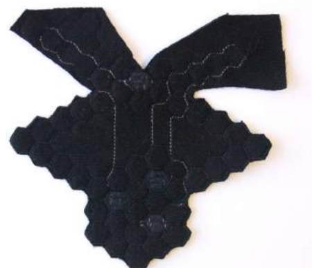
Figure 4.43 - Scaled down hexagon brace after being cut out
