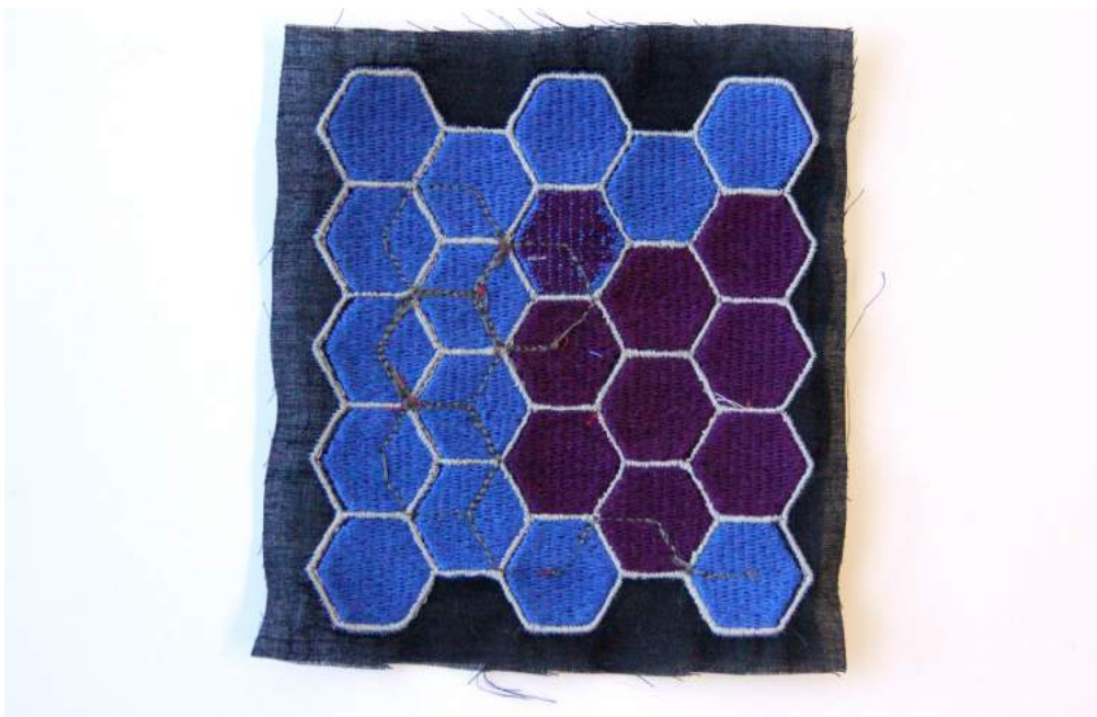
Figure 4.21 -Hexagonal outline and fill with some conductive thread stitch created with a CNC sewing machine
