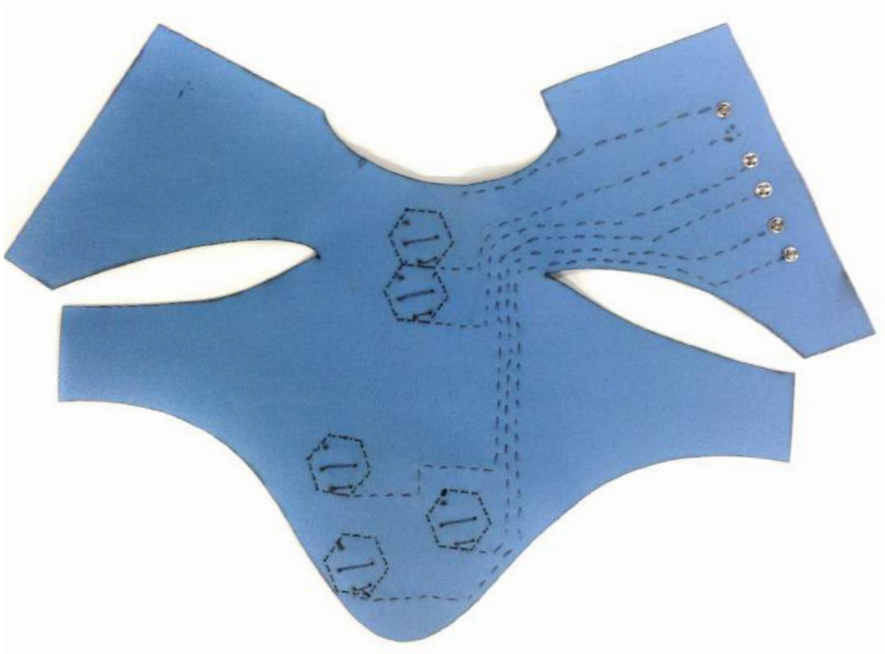
Figure 4.10 - Ankle brace with five sensors
