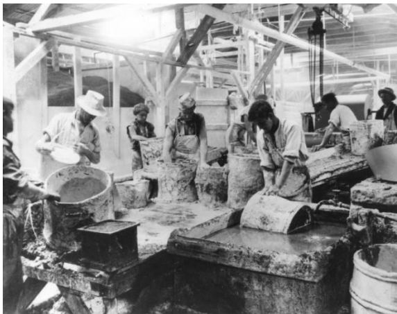
Figure 90: Workers in NZ Wallboard factory mixing plaster by hand, 1927
