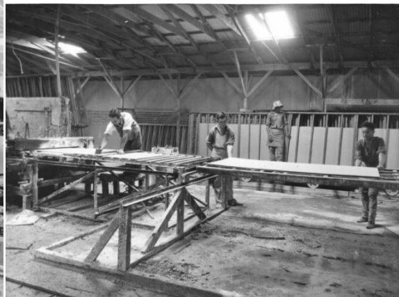
Figure 91: Hand cutting to untrimmed lengths to load in to tunnel drier 1927
