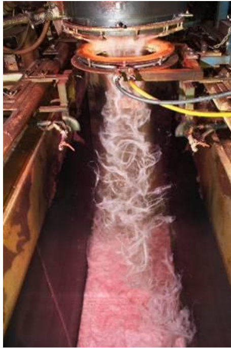
Figure 112: Glass Fiberizing Process
