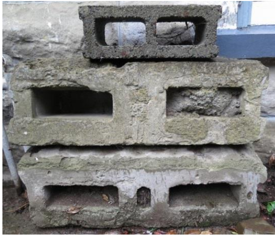
Figure 124: Blocks from Lyall Bay House. Internal block on top
