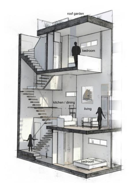
Fig. 5.38 Apartment 'A' sectional perspective.
