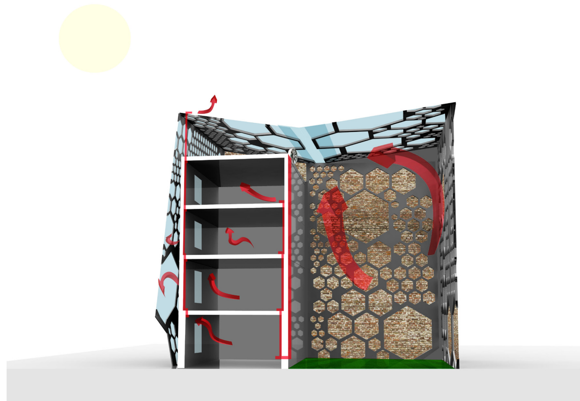
FIGURE 39: Heat from the sun is collected in the apiary. A fan then distributes this heat throughout the Edward Building when needed. This helps reduce reliance on electrical heating. Image by author, 2011.
