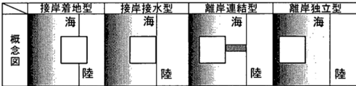
↑ Figure 2-14: 4 type of relationship between building and coastal land From, left to right, 1) Right on the shoreline; 2) Next to existing dry land; 3) Alongside pier or connected via access bridge; 4) Island type with no physical connection. Source: Kuroyanagi, A., & Sasaki, R., Exterior Composition of the Oceanic Architecture with a Plane Form , Journal of Architecture, Planning and Environmental Engineering, No. 546, (Tokyo: AIJ, 2001), pp. 317, http://ci.nii.ac.jp/ , accessed on 06/08/10.
