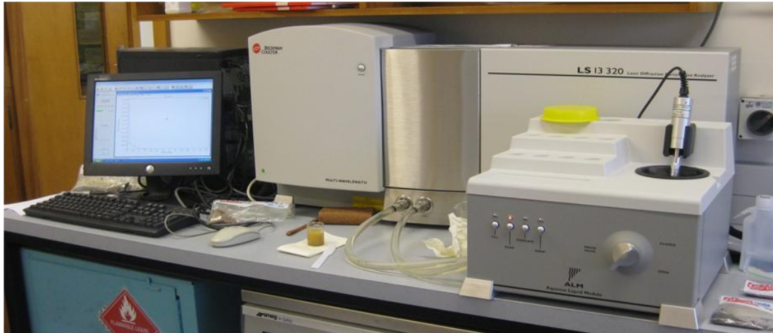
Figure 24. Beckman Coulter LS 13 320 – Laser Particle Sizer Victoria University Water Quality Laboratory.
