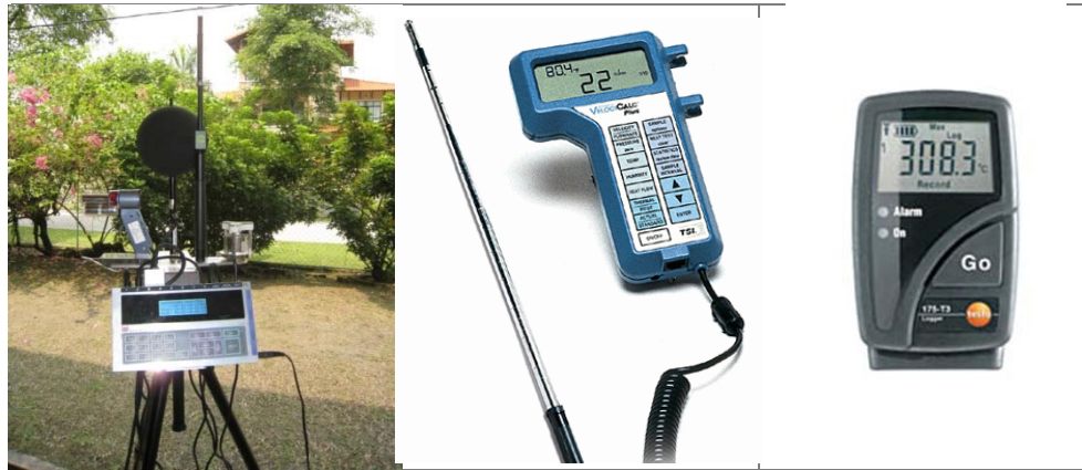
Figure 3.8. Babuc A (left), mobile TSI VelociCalc Plus Meters (middle), and electronic Mini Thermohygrograph (right)
