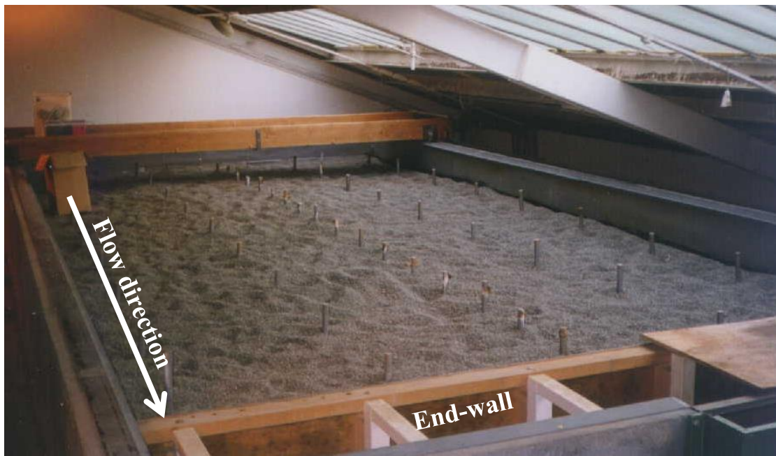
Figure 2-4: Heterogeneous artificial aquifer and monitoring wells (photo sourced from ESR archive)
