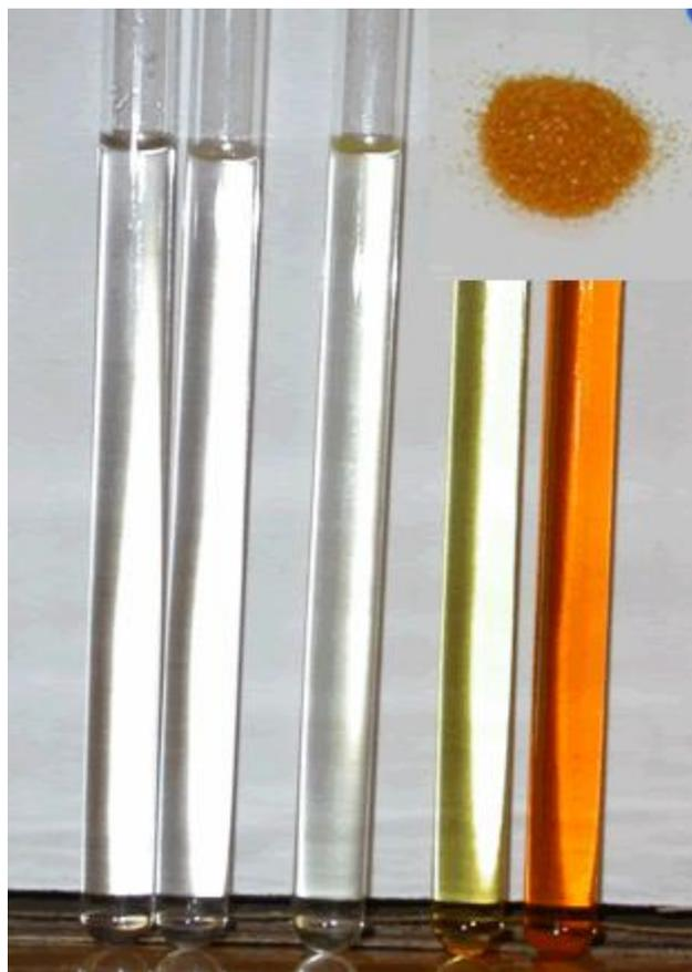
Figure 27. Precursor solution containing different ratios of oleylamine to oleic acid and  $[\text{PdCl}_2(\text{NCMe})_2]$  in powder form (inset).
