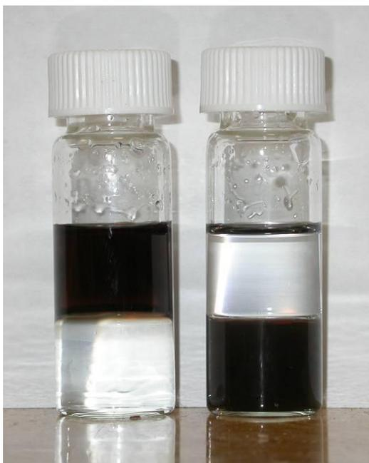
Figure 26. OLA capped PbS nanoparticles suspended in hexane layer (left) and TGA capped PbS nanoparticles suspended in aqueous layer (right).
