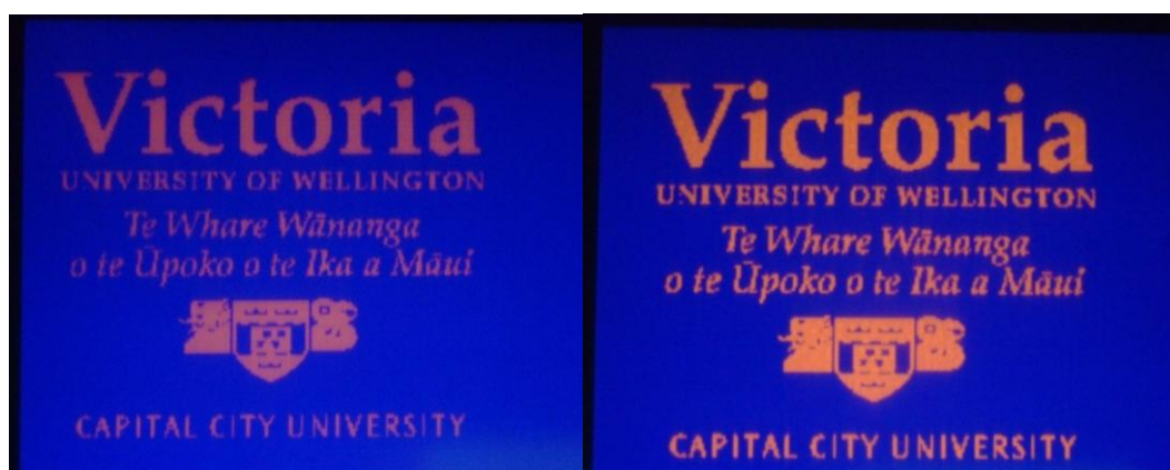
Figure 6.8. Comparison between images printed using 1 layer (left) and 2 layers (right) of \text{ZnS:Mn}^{2+} quantum dots. Viewed under UV light.
