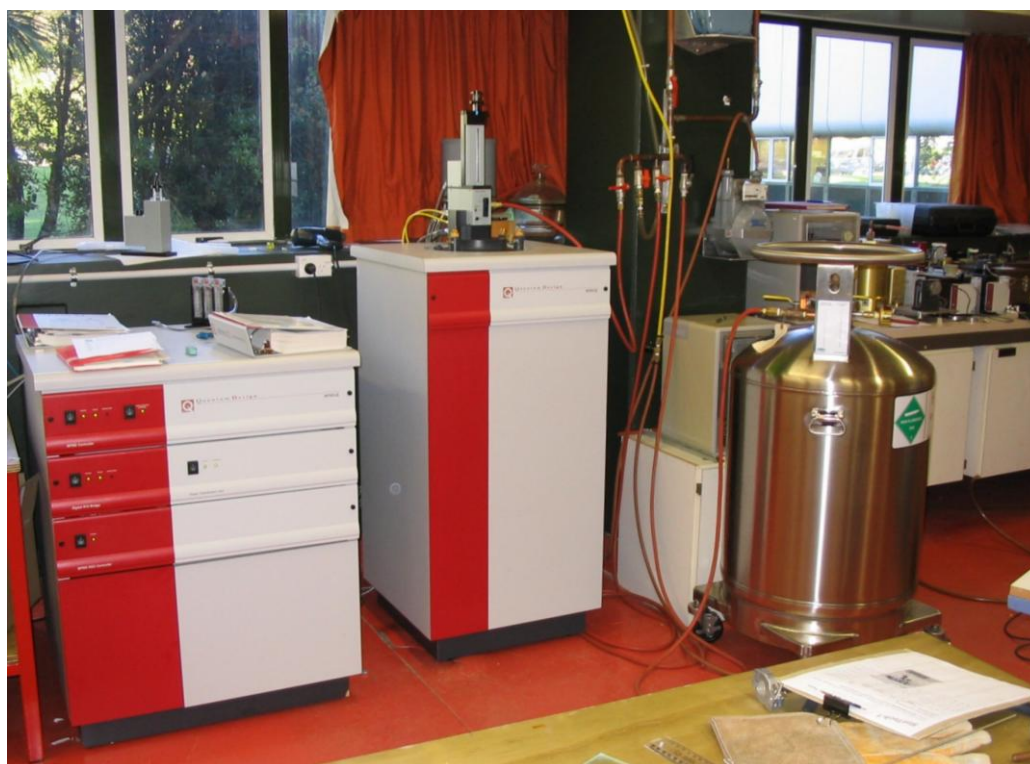
Figure 2.7. Quantum Design MPMS SQUID Magnetometer, housed at Industrial Research Ltd.
