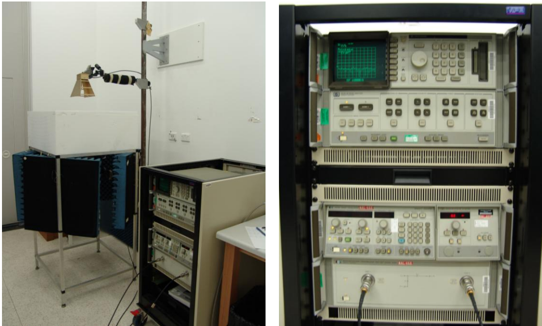
Figure 2.4. Photographs of the experimental set-up for free space measurements.
