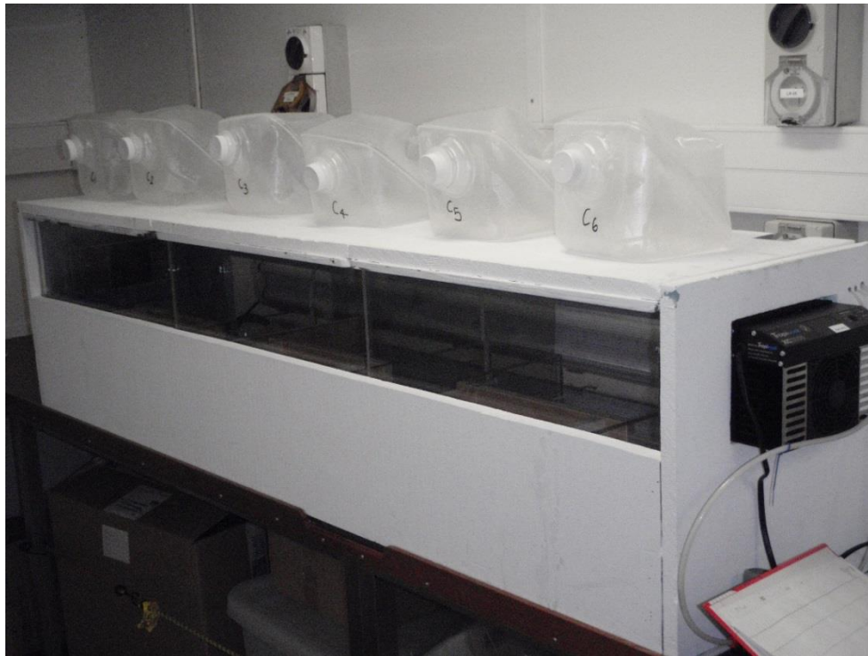
Fig. 2.4. External view of an incubation chamber on board the NIWA research vessel Tangaroa . Six empty cubitainers sit ready to be filled. To the right, a temperature controller unit is positioned inside the wall of the incubator
