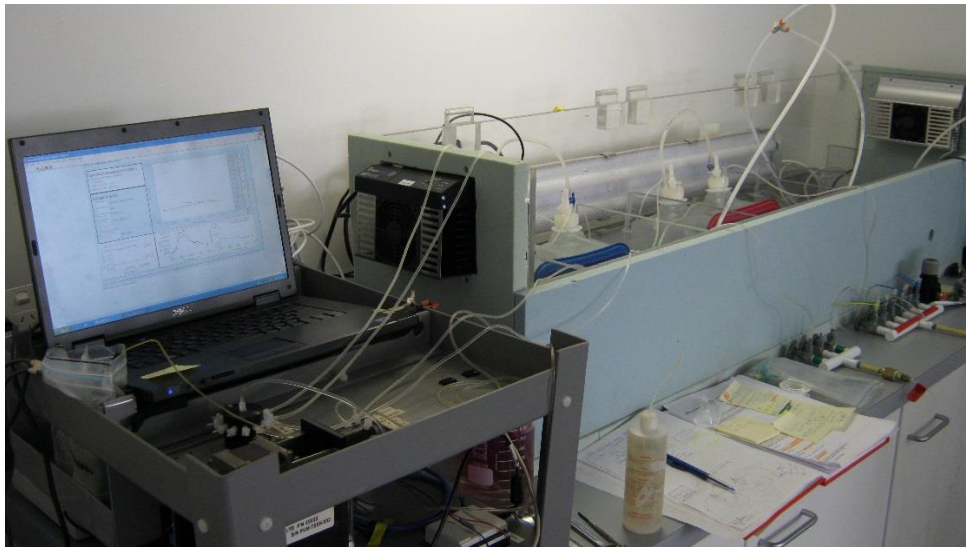
Fig. 2.3. Automated pH spectrophotometer taking pH measurements from trial seawater samples, as in Law et al. (2012)
