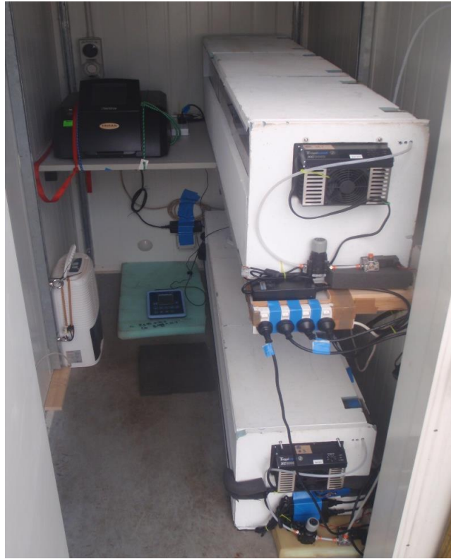
Fig. 6.4. Experimental set-up in the temperature controlled container. Two white incubation chambers are stacked on the right side, the black fluorescent plate reader can be seen raised on the bench, while the pH meter is situated on the container floor
