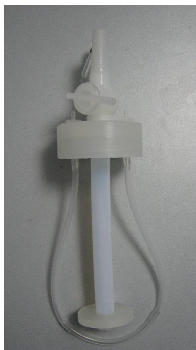
Fig. 2.2. Custom made nylon screw-cap and valve, permeable silicon tubing loop hangs below
