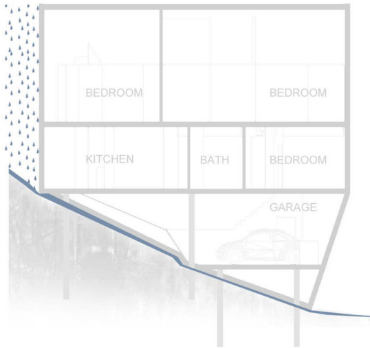
Figure 79: Diagram demonstrating house sitting slightly above ground to ensure natural water course unaffected by building - Author's own
