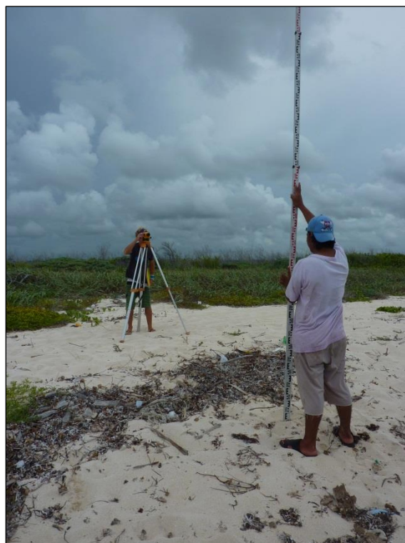
Figure 4-1: Across-shore beach profile surveying using a Sokkia B20 Automatic engineer's level.
