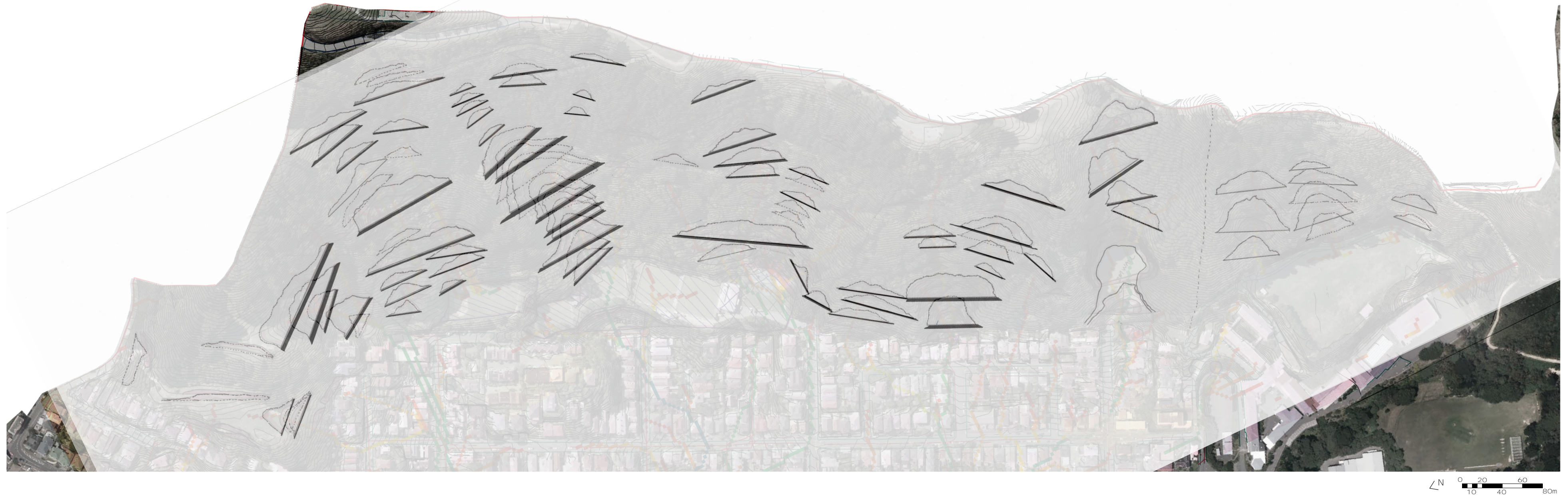
Figure 122: Straight dam walls across important detention areas - using the assumption that for 1 meter depth of water = 0.25m dam wall thickness (Author; Koordinates Ltd.; TerraMetrics and Google)
