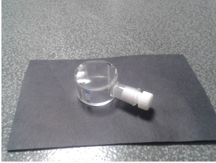
Figure 5.6: Quartz cell used for the determination of the differential Raman cross section of the A_g(2) mode of \text{C}_{60} at 633 nm.
