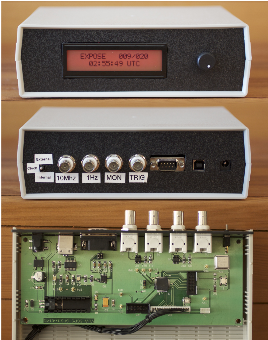
Figure 2.12: The Puoko-nui timer unit provides precise and flexible timing control. The unit connects to a GPS receiver (currently supporting both a Trimble Thunderbolt and a legacy Magellan receiver) via a serial RS232 connection and coaxial cables carrying 1 Hz and (optional) 10 MHz pulse trains. The RS232 output provides absolute time information each second via an ASCII-coded string, and both coaxial signals provide edge-aligned pulses synchronised to GPS time. Coaxial cables to the camera provide an output for frame-transfer triggers and an input for status monitoring. A selector switch allows the microcontroller clock to be switched between the 10 MHz pulse train and an internal oscillator.
