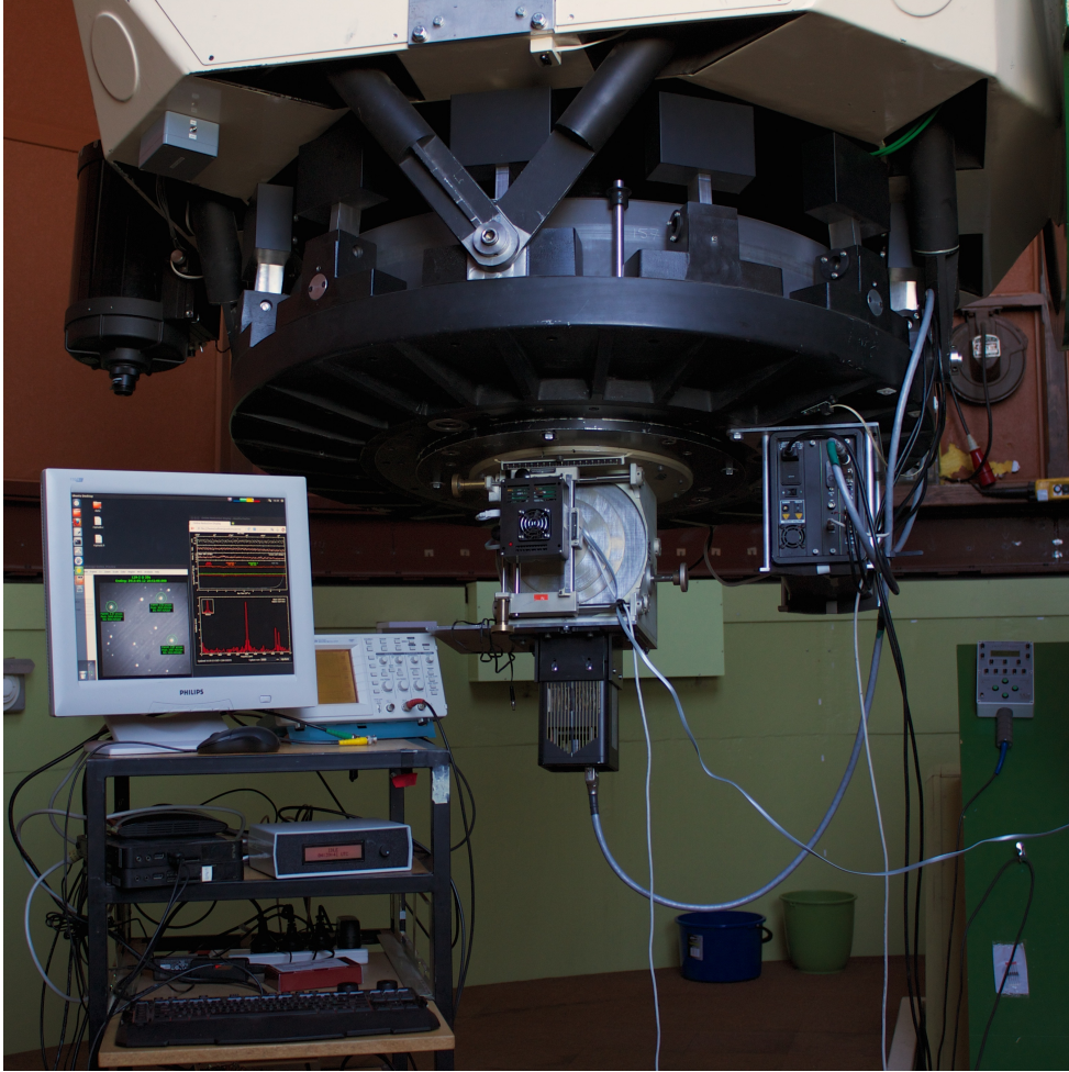
Figure 2.5: Puoko-nui South mounted on the 1.0 m McLellan telescope at MJUO.
