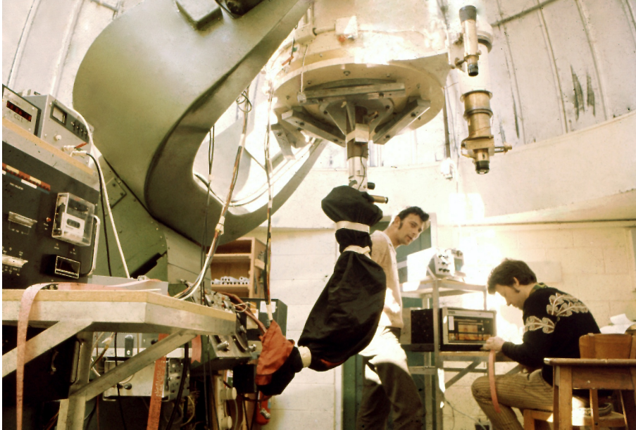
Figure 2.1: DJS and Mike Clark with the VUW single-channel photometer mounted on the 0.6 m Optical Craftsman telescope at MJUO during the late 1970's.
