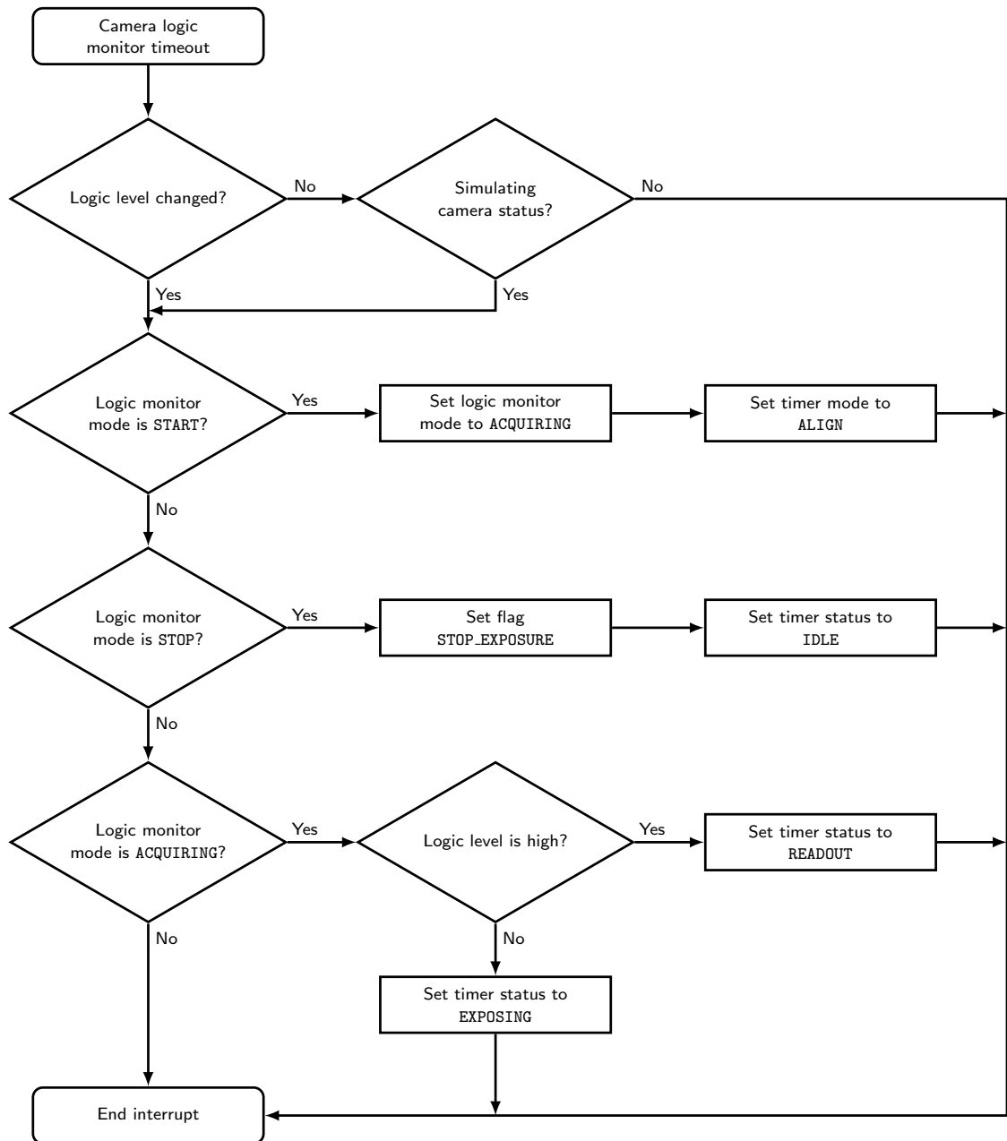
Figure B.5: A block diagram showing the camera monitoring logic.
