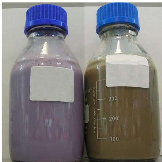
Figure 5.1: Picture nanogold (left) and nanosilver (right) hybrid polyurethane K5000 paint materials containing 0.1 wt % of \text{Au}^{3+} / \text{Ag}^{+} .
