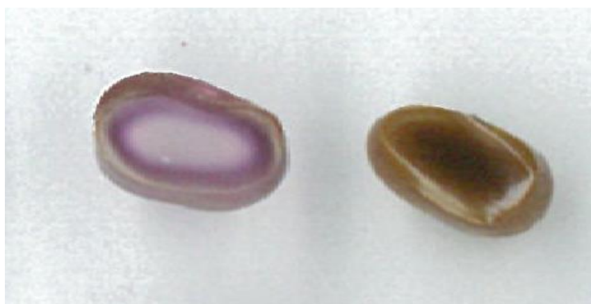
Figure 3.28: Photographs of sliced cross sections of the PU-b-50Au (left) and PU-b-500Au (right) samples.
