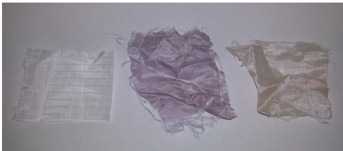
Figure 4.4: Photograph of the untreated PET sail cloth, PET-50Au and PET-50Ag samples (from left to right).
