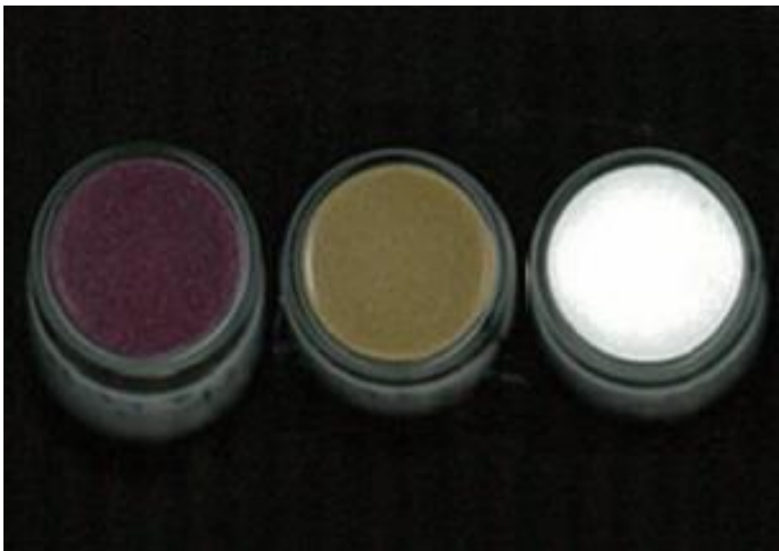
Figure 4.5: Photograph of the NH2-500Au, NH2-500Ag and untreated NH2 sorbent material samples (from left to right).
