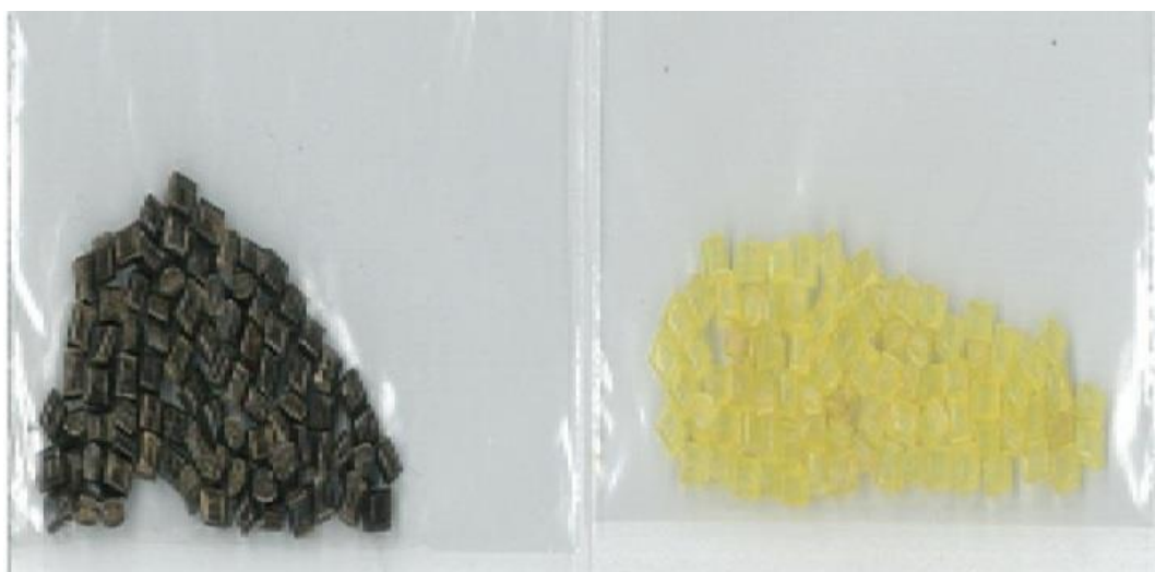
Figure 3.57: Photographs of the Ny-b-500Au beads (left) and the beads prepared via the same method but with a changed pH value of 1.4 (right).
