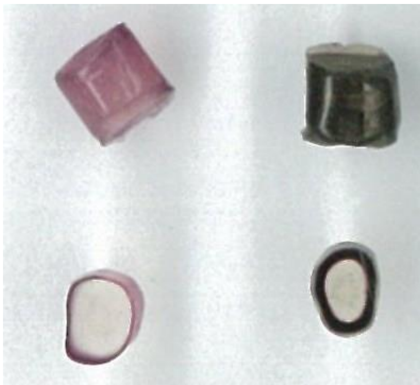
Figure 3.36: Photographs of Ny-b-50Au (left) and Ny-b-500Au (right) samples with their respective cross sections below.
