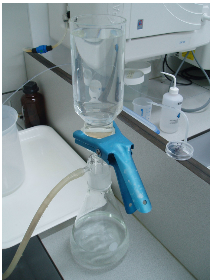
Figure 3.2: Millipore vacuum filtration system showing filtered sediment (tan colour) on filter in centre of unit.
