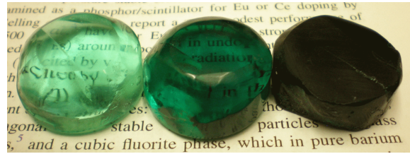
Figure 9.3: Photograph of \text{CaF}_2\text{:Sm} samples for various samarium dopant concentrations. The concentrations are 0.01 %, 0.1 % and 1 % from left to right.
