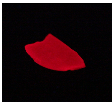
Figure 7.6: A sample showing strong red photoluminescence under 365 nm excitation from a UV mineral lamp.
