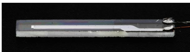
Figure 5.3: A finished OLED with a patterned ITO anode, PEDOT:PSS and PFO layers, and an Al/Ag cathode.
