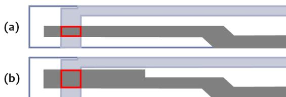
Figure 5.11: Top view schematic following Figure 5.2, showing the two different cathode patterns. The ITO anode pattern underneath is for an active area of 2 mm length. Active areas (bordered in red) are of (a) 1 mm width (b) 2 mm width.
