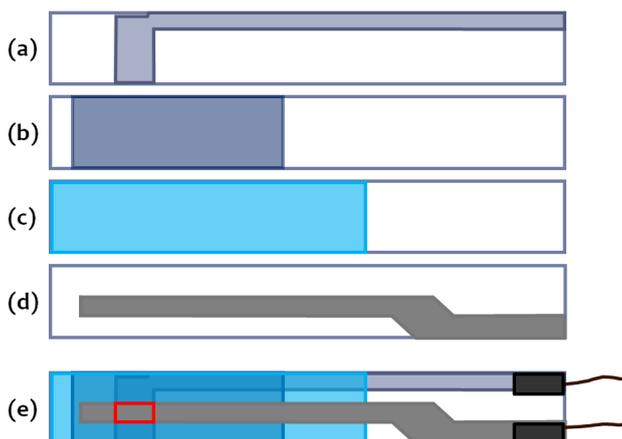
Figure 5.2: Top view of the device structure. (a) 4 mm  $\times$  25 mm glass substrate with patterned ITO electrode. (b) Spin-coated hole-transporting layer. (c) Spin-coated light-emitting layer. (d) Thermally-evaporated metal cathode. (e) The final structure with the 2 mm  $\times$  1 mm active area highlighted by a red bordered rectangle.
