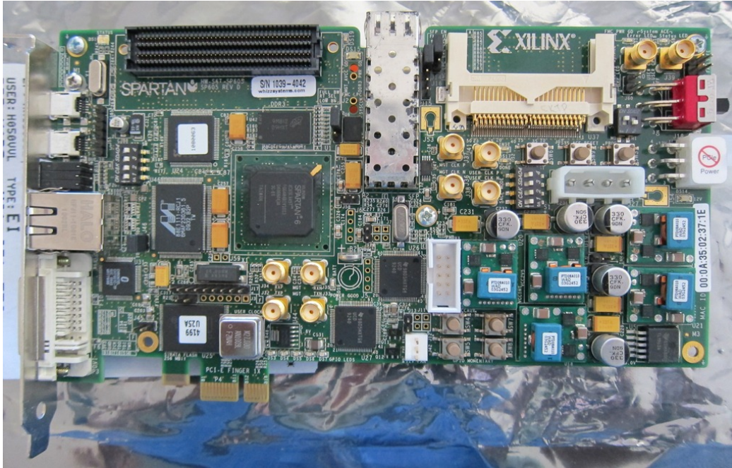
Figure 4.3: Xilinx PCI Express Spartan-6 Connectivity Kit Board - The SP605
