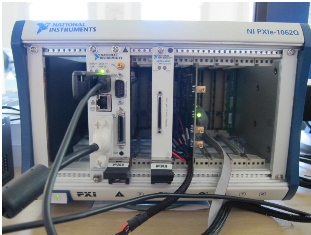
Figure 4.2: Designed PXI Express Peripheral Module installed in the NI PXIe-1062Q Chassis
