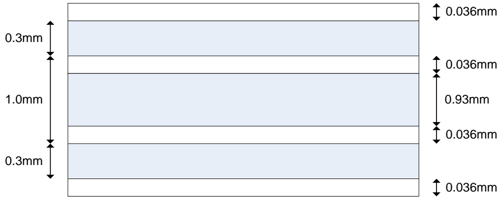
Figure 3.32: Structure of standard 4 Layer PCB
