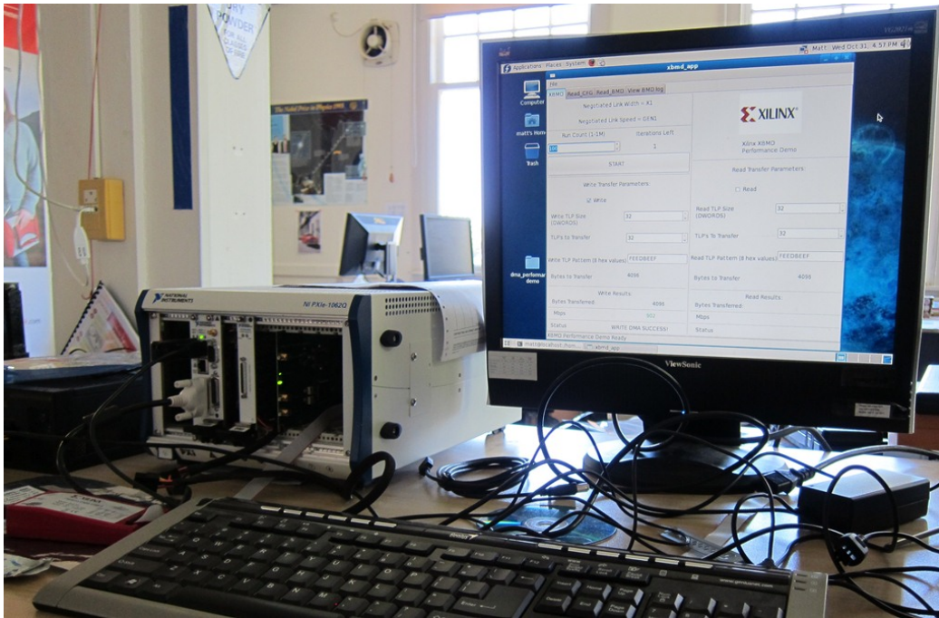
Figure 4.16: PXI Express system installed with PXI Express Peripheral Module running example application
