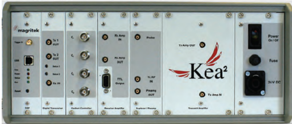
Figure 2.1: An example of a Magritek Spectrometer - The Kea 2 [4]
