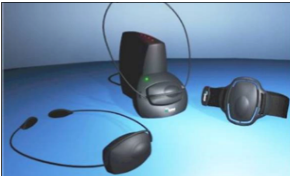
Figure 5: EMG biometric and gyro-based position controller (arm bands, headbands and base) used in (Tanaka and Knapp 2002)
