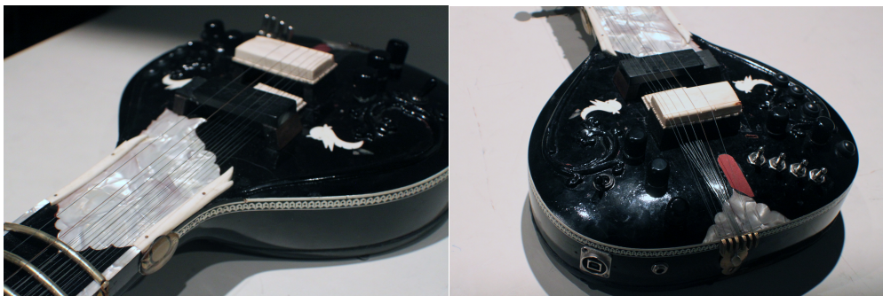
Figure 9: Esitar sensor systems, close up of thumb sensor (left), and usb, standard audio jack, knobs, buttons, and switches (right)
