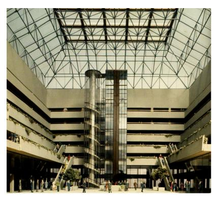
Figure 2.9 Atrium space (model) to proposed civic centre, Liverpool, 1967. The early date of this atrium proposal indicates that Portman was not the only architect exploring atria at this time. As can be seen, this atrium dealt with sunlight, security, circulation, visual and physical connectivity. Increased access to fresh air is also assumed. Architect: Colin St John Wilson. *Source: Stonehouse, p418.*
