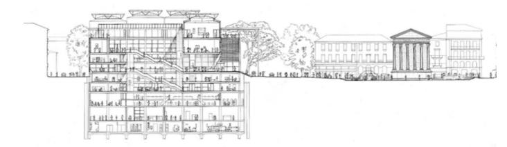
**Figure 5.2.3 Cross section through Carré d'Art.** This section shows the overall relation of the building to the urban environment, including the Roman temple. An enlarged version of the section appears in 5.2.16 *Source: Foster and Partners*
