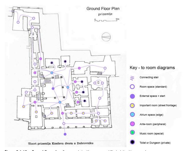
$\textbf{Figure 5.1.13-Ground floor plan.} \ \textbf{Gamma analysis with room permeability} \ / \ \textbf{relationships mapped}.$
