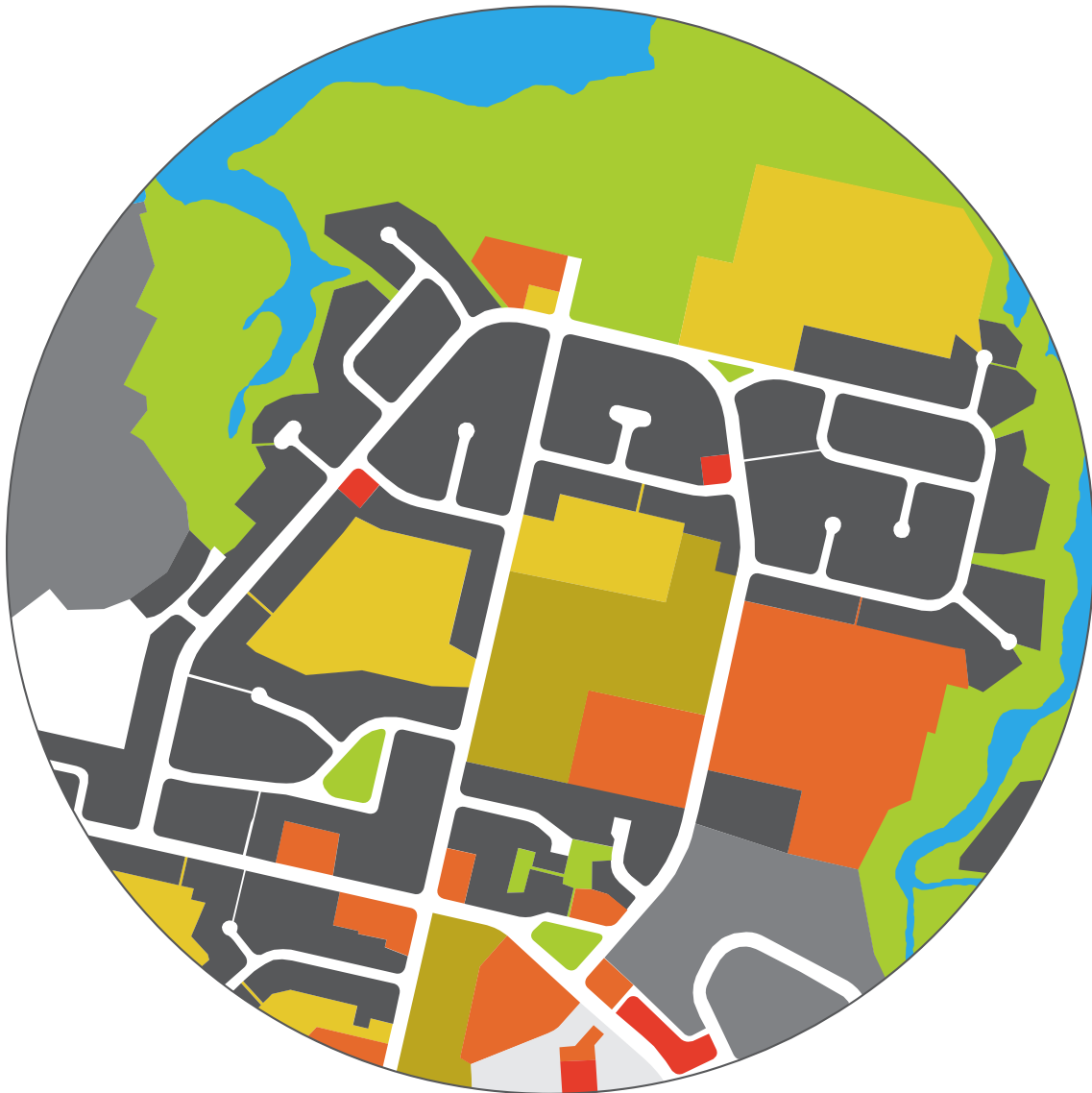
Figure 97. Pre-intervention suburban diagram illustrating the design case study area's large superblocks and poor connectivity. Note how the schools, tertiary institution, and enveloping public reserve integrate poorly with the area.
