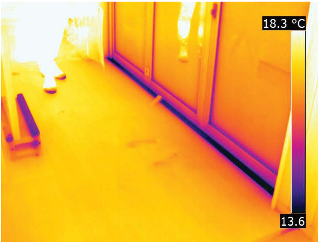
Figure 88: Faulty seal at the base of the bifold doors (Source: Image courtesy of BRANZ)
