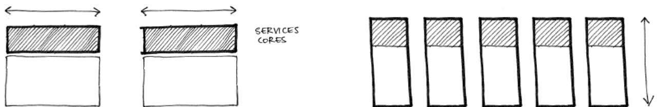
Figure 4.1 Plan diagrams showing a fundamental change in the structural makeup of the building from longitudinal to lateral.
