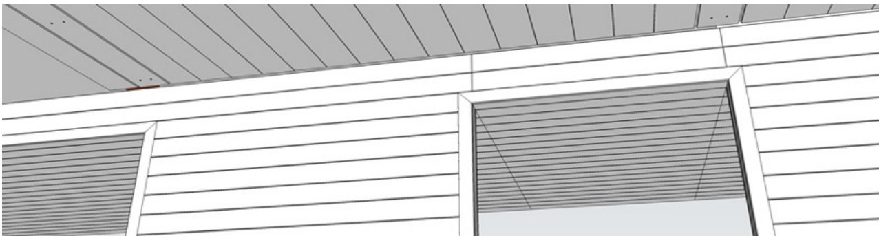
Figure 8.17 Lining up a removable hatch in the bulkhead space with the door and module join
