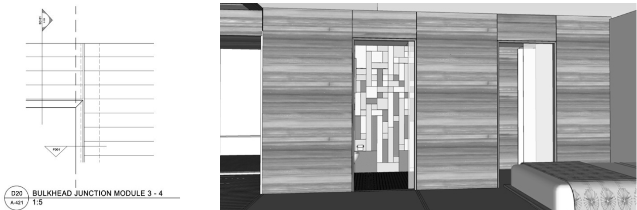
Figure 8.15 Trialling a negative-detailed ‘panel’ above the doorways and central services space. This did not achieve the look the design team desired, and its construction allowed little tolerance in the assembly stage.
