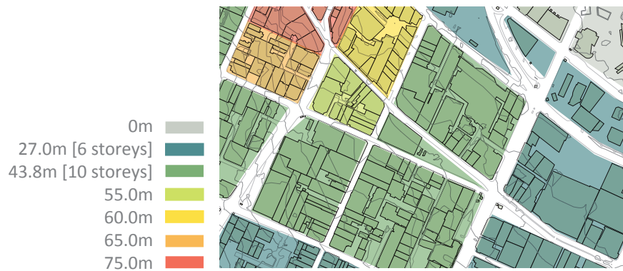
Figure 4.8. Building height restrictions of site and surrounding area. The site exists at a location where Wellington's 'low' city area of Te Aro begins to increase in height towards the 'high' city area of the central business district
