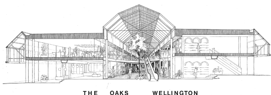
Figure 4.16. Sectional perspective of The Oaks retail complex as it was proposed in 1980. The central atrium space has since been enclosed.
