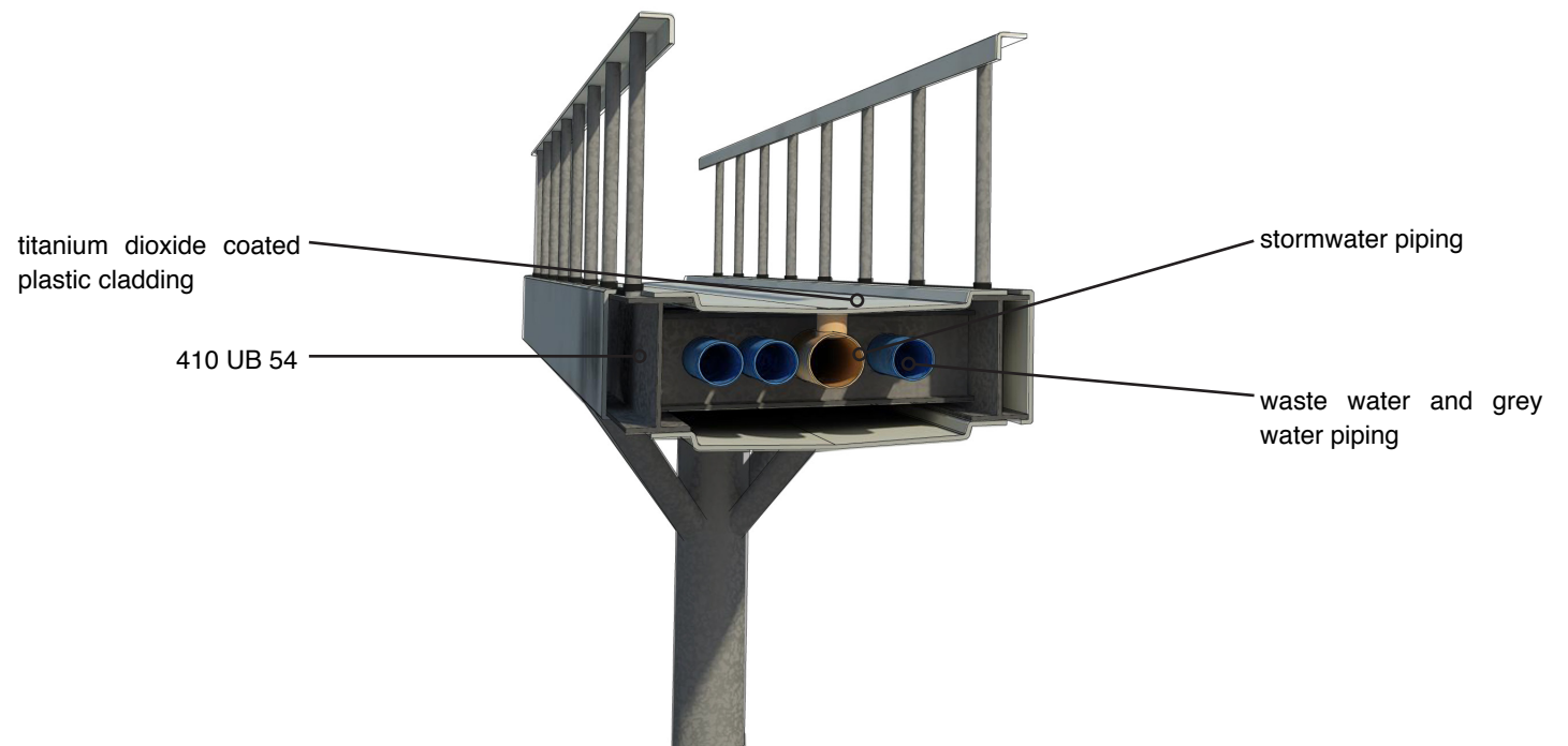
Figure 84: Hexagonal structural framework detail (stage two). The frame is now used for access. It is fully clad in panels that use a TiO 2 coating based on that of Prosolve panels. Handrails attach to the structural steel and services run through the centre.
