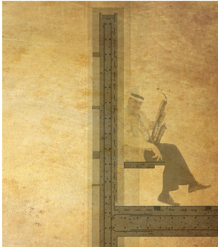
FIGURE 48: SECTION THROUGH WATER TRACE SEATING. STEEL REINFORCING IS SET INTO RAIN GROOVE ALLOWING RUST STAINS TO BE DIRECTED
