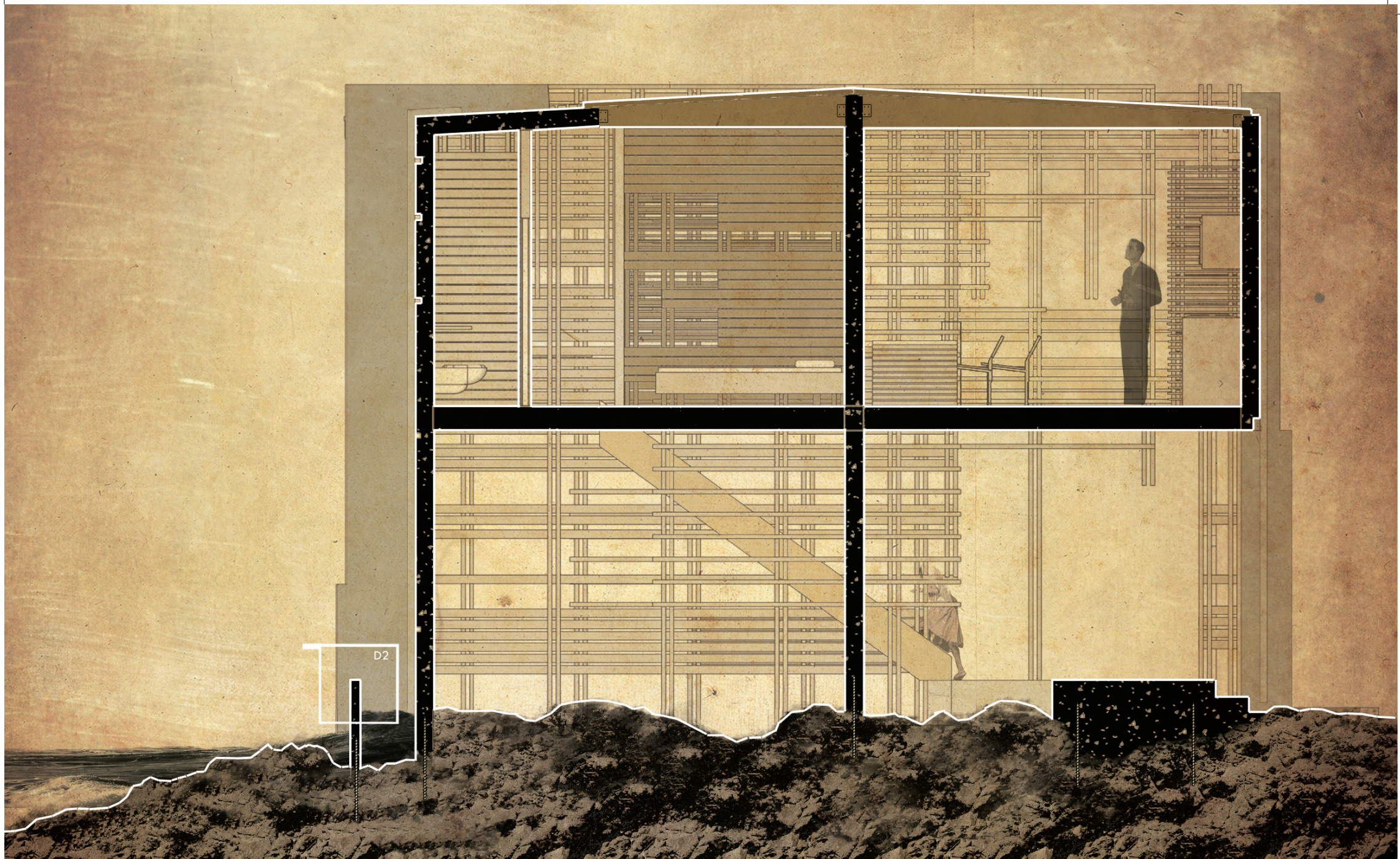
FIGURE 36: SECTION B -B PUBLIC ACCESS IS MAINTAINED UNDERNEATH BUILDING WITH MINIMIZED EFFECT ON EXISTING ENVIRONMENT. ON THE LEFT HAND SIDE, THE CONCRETE WALL WRAPS OVER TO FORM A PARTIAL ROOF. THIS EMPHASIZES ITS USE AS A PROTECTIVE ELEMENT AS IT IS EXPERIENCED FROM THE INTERIOR ALSO. AS DISCUSSED IN CHAPTER ONE, ALL MATERIALS EXPRESS THEIR TRUE IDENTITY ALLOWING THE USERS TO FEEL COMFORTABLE INTERACTING WITH THEM.
