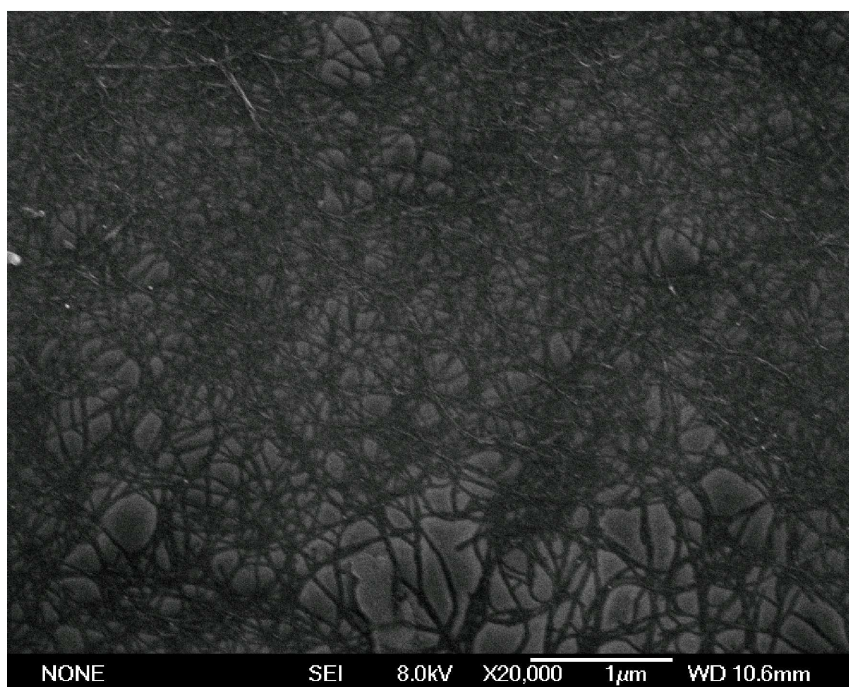
Figure 4.10: SEM image of a film annealed at 300 °C.
