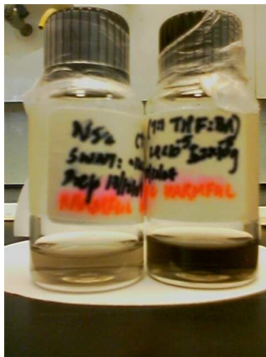
Figure 4.3: Two dispersions of different SWNT concentrations prepared with a 7:1 solvent to surfactant ratio. The solution on the left was prepared according the amounts described in Section 4.1.3 while the one on the left was made with twice the initial amount of SWNTs.
