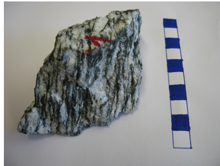
Figure 3.4: Photography of a rock sample of the granitic intrusion east of Ralfes Knob presenting important foliation. Its wet density is 2.66 \text{ Mg/m}^3 . Each division is 1 cm wide. Courtesy of Mark Rattenbury.
