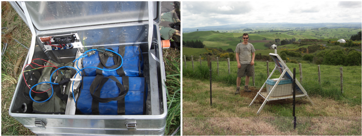
FIGURE 4.2 Station set up for broadband recorder. Left: The box for the digitiser containing three 12 V batteries. Right: The fenced station with solar panel and GPS unit.
