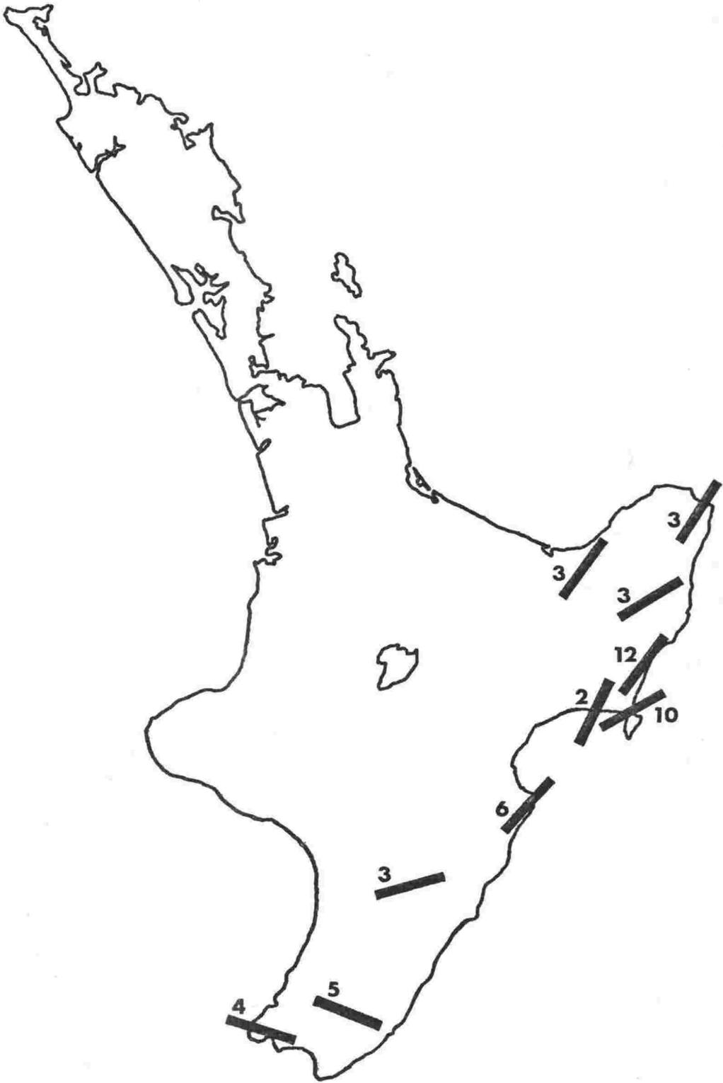
Figure 6.6 Shear strain components from retriangulation data for the period after 1931, after Walcott (1978b). The numbers are rates of shear strain in units of  $10^{-7}/\text{yr}$ , and the bars mark the direction of the principal axis of horizontal compression.
