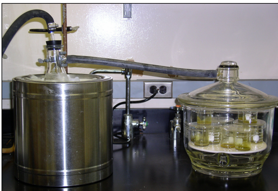
Figure 3.4: Vacuum drying set-up for drying samples following the removal of carbonate.
