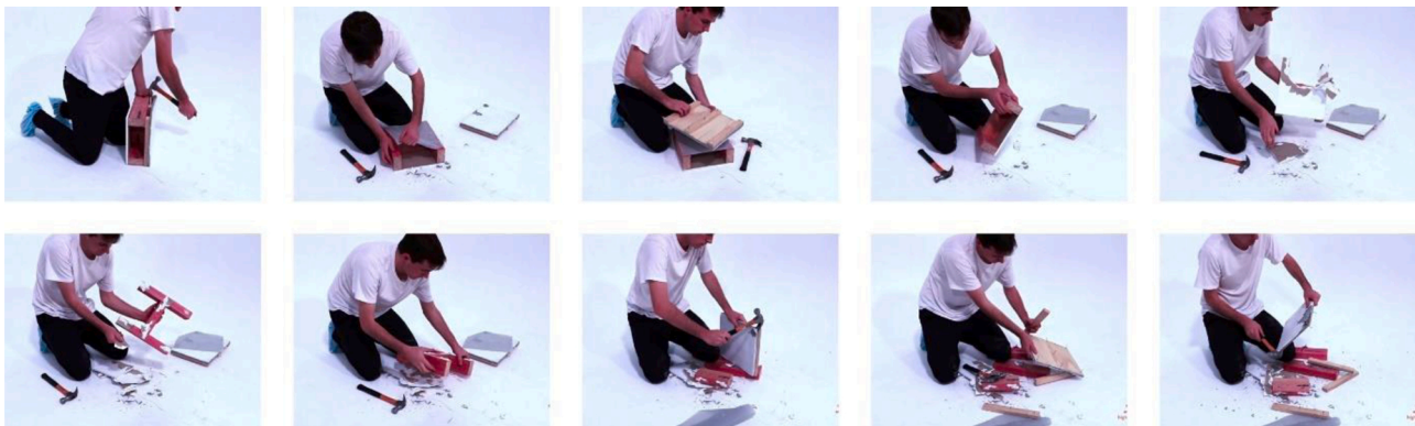
Fig. 3. A deconstruction sequence (left to right, top to bottom) showing destructive removal of the 'stucco' plaster and paint cladding and building wrap. This is followed by destructive removal of the plasterboard internal wall lining. Finally separation of the treated timber cavity battens from the rear of the stucco assembly is attempted.
