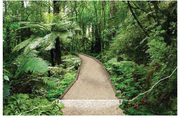
Figure 258. Path Type 1 - Crushed Gravel. 2m Wide. Walking and Cycling
