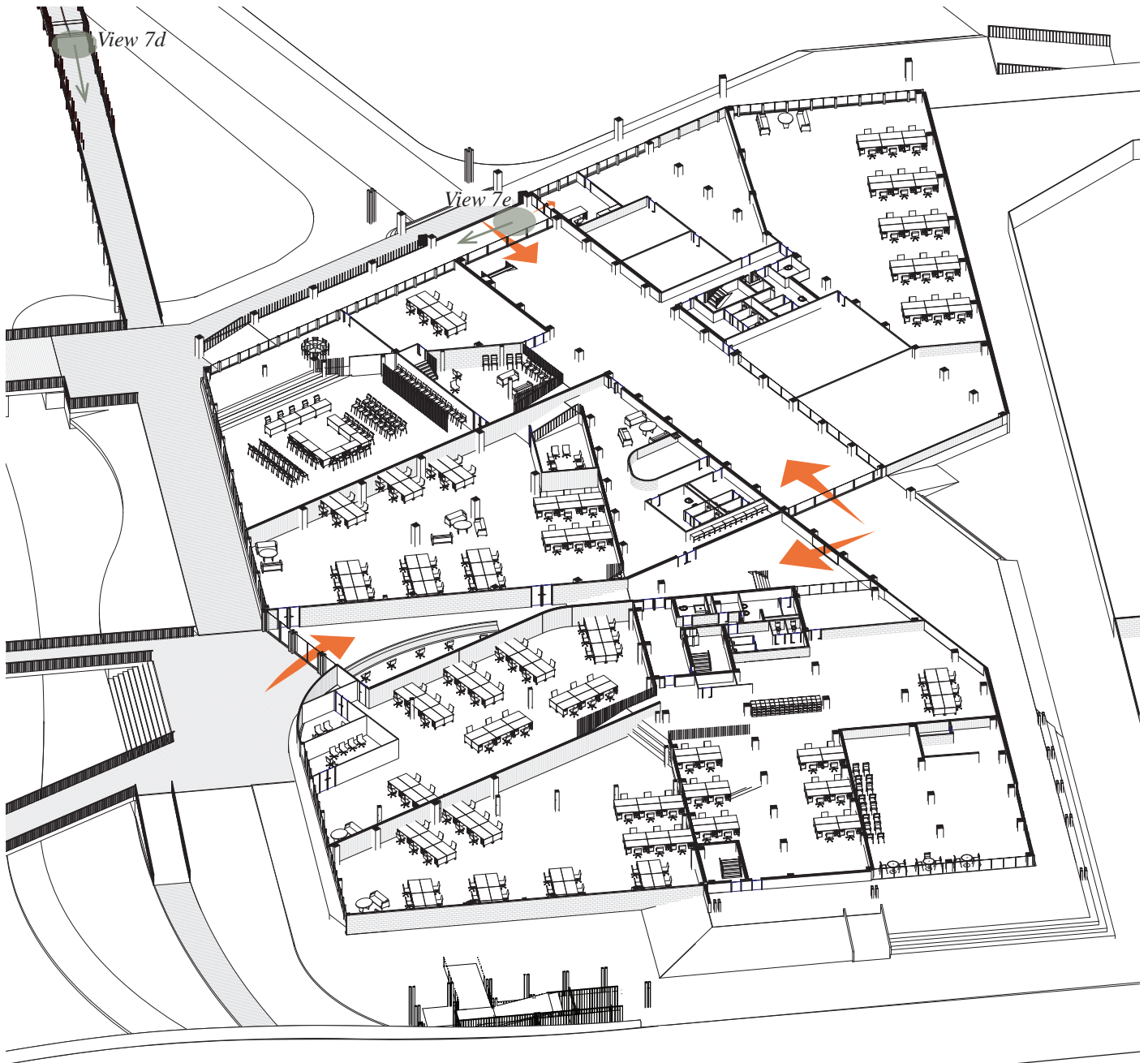
Fig7.35. Isometric plan showing main building entrances and buildings edge condition.
