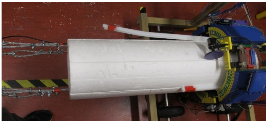
Figure 12 Experimental setup for testing mock pre-stressed power pole with eddy current testing system
