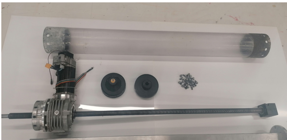
Fig. 59: Robotic Arm & Clay extruder attachment Fig. 60: Clay extruder parts
