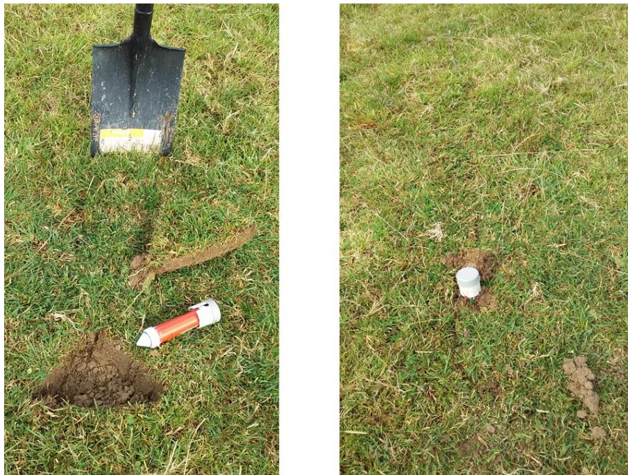
Figure A5: Cu/CuSO 4 electrode prepared to be installed and post installation.
