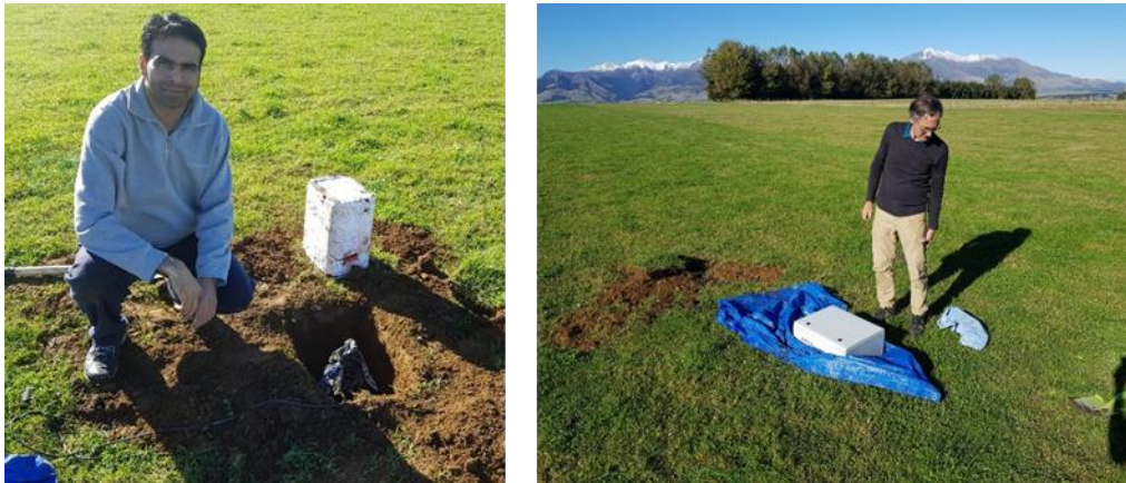
Figure 2. 18: Left hand panel: magnetometer hole with the author sitting beside it. Right hand panel: data logger for recording electric and magnetic fields. The electrodes for electric field measurements are spread ~50 m apart and are not shown in these pictures.
