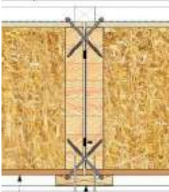
ModCell® panel to panel connection (plan)
