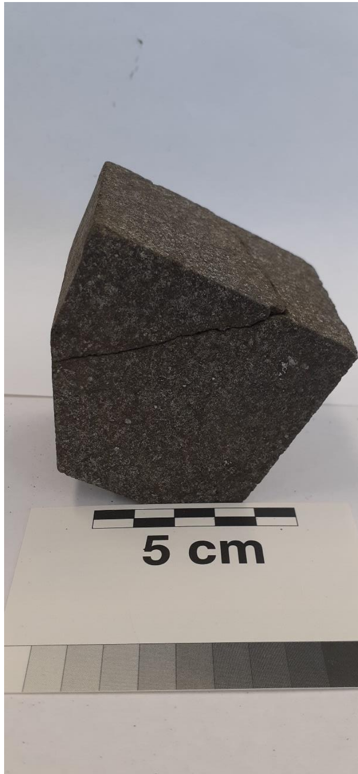
Figure 4-13: Cut block hand sample of TAN1213 10-10 showing colour, texture, and grainsize
