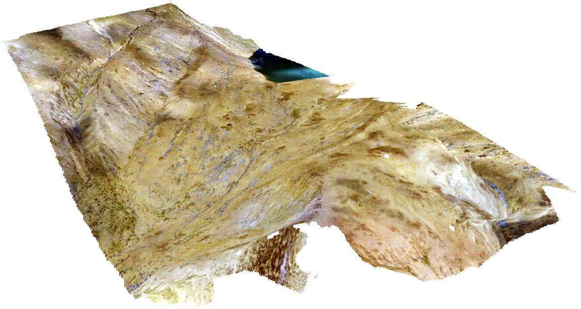
Figure 3.1: 3D model produced by compilation of drone photographs using Structure from Motion technology. Perspective looking northwest, up valley towards the cirque lake. Model has 25 cm resolution.
