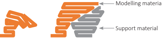
Figure 54. Author, Use support material to increase the printability
