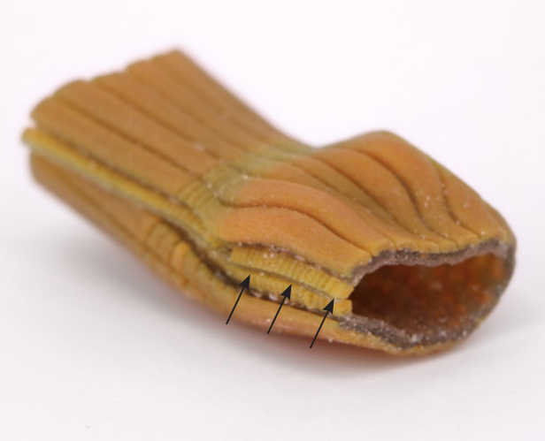
Figure 51. Author, Split of the zip in a previous 1:3.3 scaled prototype
