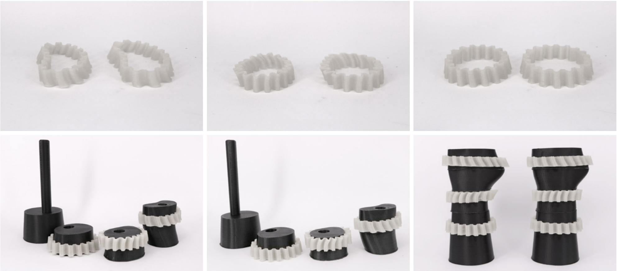
Figure 46. Author, Final prototypes printed with the new materials programmed on the two moulds
